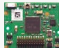
Wireless ZigBee® Pro module / Green Com card.
